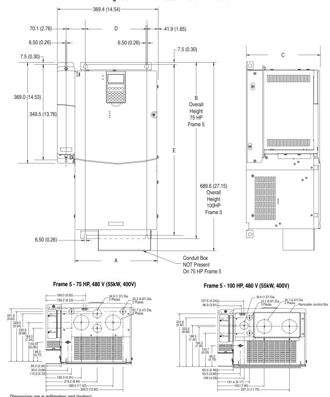
Figure 5 PowerFlex 700S Frame 5 Dimensions
