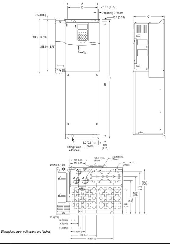
Figure 4 PowerFlex 700S Frame 4 Dimensions
