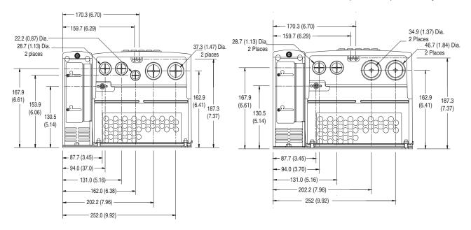
Dimensions are in millimeters and (inches)
