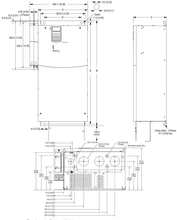
Figure 6 PowerFlex 700S Frame 6 Dimensions
