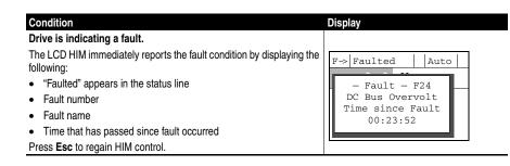
**Manually Clearing Faults**
